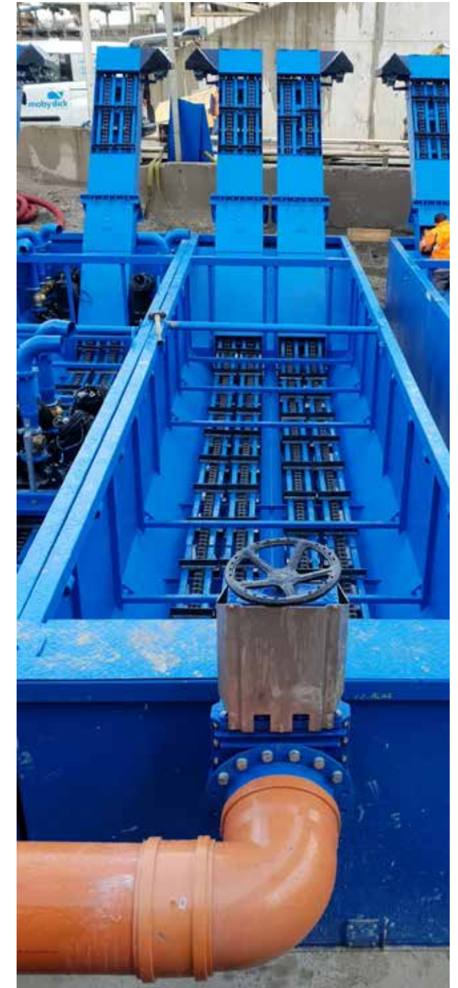
Recyclingtank 50DCC Doppelkratzförderer-Technologie Recycling tank 50DCC double scraper conveyor technology
