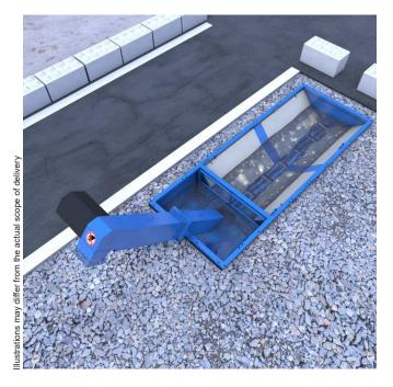
The washed-off solids settle out in the recycling tank. The integrated scraper conveyor conveys settled sludge from the recycling tank. The water is fed via the overflow wall with sieve insert into the pump chamber. It is recommended to use the MobyDos Compact flocculant dosing system (optional).
