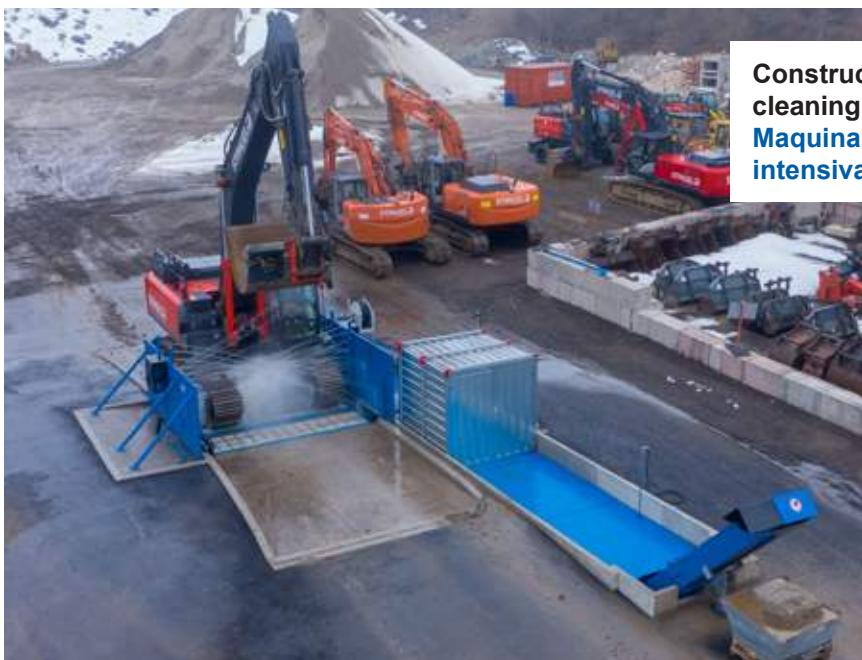
**Construction machines: Intensive primary cleaning in just a few minutes**
