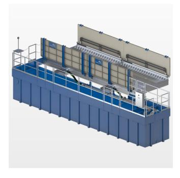
In all MobyDick wheel washing systems the water is circulated in a closed circuit. Water treatment is via sedimentation in the recycling tank. Sedimentation can be accelerated by adding a flocculant. The solids that settle out in the recycling tank should be extracted with an excavator or suctioned out with a suction vehicle at regular intervals (depending on how frequently the system is used).
