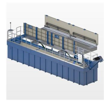
In all MobyDick wheel washing systems the water is circulated in a closed circuit. Water treatment is via sedimentation in the recycling tank. Sedimentation can be accelerated by adding a flocculant. Settled solids are continuously conveyed out of the recycling tank by the scraper conveyor.
