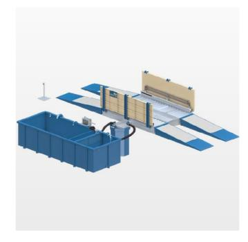
In all MobyDick wheel washing systems the water is circulated in a closed circuit. Water treatment is via sedimentation in the recycling tank. Sedimentation can be accelerated by adding a flocculant. The solids that settle out in the recycling tank should be extracted with an excavator or suctioned out with a suction vehicle at regular intervals (depending on how frequently the system is used).
