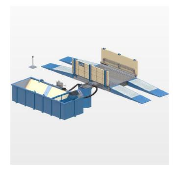
In all MobyDick wheel washing systems the water is circulated in a closed circuit. Water treatment is via sedimentation in the recycling tank. Sedimentation can be accelerated by adding a flocculant. Settled solids are continuously conveyed out of the recycling tank by the scraper conveyor.
